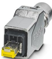
RJ45 connector, degree of protection: IP65/IP67, number of positions: 8, 10 Gbps, CAT6<sub>A</sub>, connection method: IDC fast connection, connection cross section: AWG 23- 22, cable outlet: straight, Ethernet
