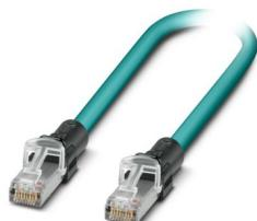
Patch cable, RJ45/IP20 straight on RJ45/IP20 straight, cable length: 3 m, number of positions: 8, 10 Gbps, CAT6<sub>A</sub>, connection cross section: AWG 26- 26, Ethernet, 4x2xAWG26/7; S/FTP, water blue RAL 5021
