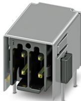
PCB headers, color: black, nominal current: 5 A, rated voltage (III/2): 160 V, contact surface: Au, contact connection type: Pin, number of positions: 2, product range: DMC 0,5/..-G1-SH-THR, pitch: 2.54 mm, mounting: THR soldering / wave soldering, solder pin [P]: 2 mm, plug-in system: COMBICON DFMC 0,5 shielded, Electrical properties: shielded, Pin connector pattern alignment: Standard, locking: shielded connection, mounting method: without, type of packaging: 24 mm wide tape, Suitable for CAT5
