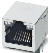
Modular RJ45 PCB connectors, 1x1 single-port, connection direction of the connector to the PCB: 90 °, Tab up, Shielded, Bicolor LED (green-yellow, green-yellow), number of positions: 8, 10 Gbps, PoE++, THT, Wave, type of packaging: Tray
