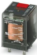
Plug-in industrial relay in basic design with power contacts, 2 changeover contacts, test button, status LED, mechanical switch position indicator, input voltage: 24 V AC
