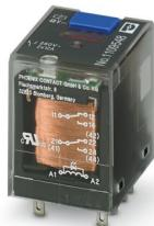
Plug-in industrial relay in basic design with power contacts, 2 changeover contacts, test button, status LED, mechanical switch position indicator, polarity A1+, A2-, input voltage: 48 V DC
