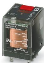
Plug-in industrial relay with power contacts, 2 changeover contacts, test button, status LED, mechanical switch position indicator, input voltage: 230 V AC
