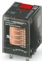
Plug-in industrial relay in basic design with power contacts, 4 changeover contacts, test key, mechanical switch position indicator, input voltage: 230 V AC
