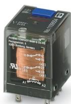
Plug-in industrial relay in basic design with power contacts, 2 changeover contacts, test button, status LED, mechanical switch position indicator, polarity A1+, A2-, input voltage: 220 V DC
