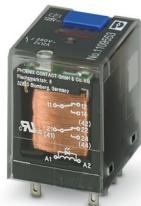
Plug-in industrial relay in basic design with power contacts, 2 changeover contacts, test button, status LED, mechanical switch position indicator, polarity A1+, A2-, input voltage: 125 V DC
