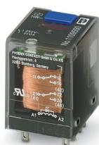
Plug-in industrial relay in basic design with power contacts, 2 changeover contacts, test button, status LED, mechanical switch position indicator, polarity A1+, A2-, input voltage: 110 V DC
