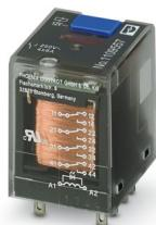
Plug-in industrial relay in basic design with power contacts, 4 changeover contacts, test button, status LED, mechanical switch position indicator, polarity A1+, A2-, input voltage: 12 V DC
