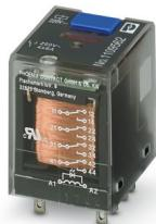
Plug-in industrial relay in basic design with power contacts, 4 changeover contacts, test button, status LED, mechanical switch position indicator, polarity A1+, A2-, input voltage: 220 V DC
