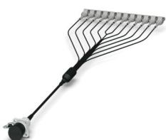
M17 series with preassembled FO socket assembly: 24-pos. M17 socket, LC duplex on the other end, 0.6 m long, multimode fiberglass G62.5/125 µm OM1, IP67 degree of protection after being inserted, fixed installation for indoor use
