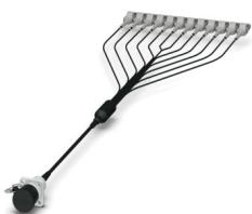
M17 series with preassembled FO socket assembly: 24-pos. M17 socket, LC duplex on the other end, 1 m long, multimode fiberglass G62.5/125 µm OM1, IP67 degree of protection after being inserted, fixed installation for indoor use
