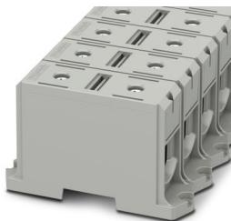
High-current terminal block, nom. voltage: 1000 V, nominal current: 380 A, number of connections: 2, number of positions: 1, connection method: Screw connection, Rated cross section: 240 mm<sup>2</sup>, cross section: 35 mm<sup>2</sup> - 240 mm<sup>2</sup>, Rated cross section: 240 mm<sup>2</sup>, cross section: 35 mm<sup>2</sup> - 240 mm<sup>2</sup>, mounting type: Screw mounting, color: gray
