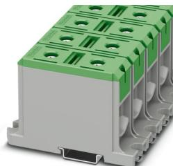
High-current terminal block, nom. voltage: 1000 V, nominal current: 290 A, number of connections: 2, number of positions: 1, connection method: Screw connection, Rated cross section: 150 mm<sup>2</sup>, cross section: 35 mm<sup>2</sup> - 150 mm<sup>2</sup>, Rated cross section: 150 mm<sup>2</sup>, cross section: 35 mm<sup>2</sup> - 150 mm<sup>2</sup>, mounting type: NS 35/15, NS 35/7,5, color: green
