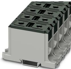
High-current terminal block, nom. voltage: 1000 V, nominal current: 220 A, number of connections: 2, number of positions: 1, connection method: Screw connection, Rated cross section: 95 mm<sup>2</sup>, cross section: 16 mm<sup>2</sup> - 95 mm<sup>2</sup>, Rated cross section: 95 mm<sup>2</sup>, cross section: 16 mm<sup>2</sup> - 95 mm<sup>2</sup>, mounting type: NS 35/15, NS 35/7,5, color: black
