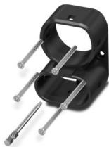
CHARX connect standard, CCS type 2, Repair kit, Accessories, housing: black, with replaceable mating face frame, with 5x M4X45 rounded head screws with Torx security drive, with special bit (867/4 IPR TORX PLUS® bit, 20 IPR x 89 mm) for insulated screwdriver, for replacement of the mating face frame of vehicle charging connectors, IEC 62196-3, The vehicle connector housing does not have to be opened in order to replace the mating face frame.
