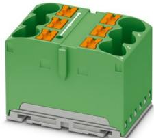
Distribution block, bridged internally, nom. voltage: 450 V, nominal current: 57 A, number of connections: 6, connection method: Push-in connection, Rated cross section: 10 mm<sup>2</sup>, cross section: 0.5 mm<sup>2</sup> - 16 mm<sup>2</sup>, mounting type: for snapping onto a DIN rail adapter, Direct mounting with flange, Free-hanging, color: green
