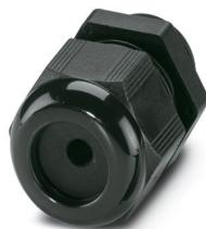
Plastic cable gland with slotted seal, for connector with pre-wired cable, IP66, M25 connection thread, clear width: 18.2 mm, outer cable diameter: 3 mm ... 6 mm
