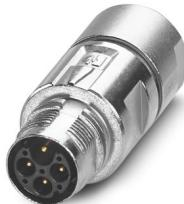
M17, Coupler connector, series: M17 PRO, straight, shielded: yes, for standard and ONECLICK fast locking system, No. of pos.: 3+PE, contact connection type: Pin, Crimp connection, cable diameter range: 3.5 mm ... 6.5 mm, Item is lead-free in accordance with RoHS II without Exemption 6c (Pb < 0.1 %)
