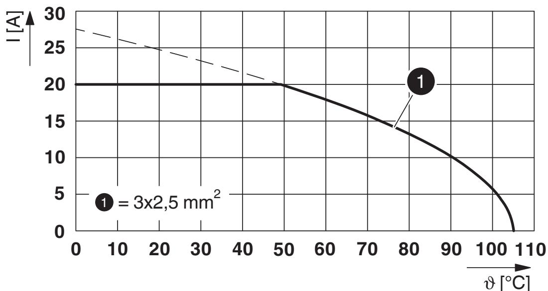
$I$  = current strength,  $\vartheta$  = ambient temperature, 3x 20 A
