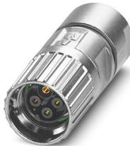
M17, Cable connector, series: M17 PRO, straight, shielded: yes, Screw locking mechanism, No. of pos.: 3+PE, contact connection type: Socket, Crimp connection, cable diameter range: 3.5 mm ... 6.5 mm, Item is lead-free in accordance with RoHS II without Exemption 6c (Pb < 0.1 %)
