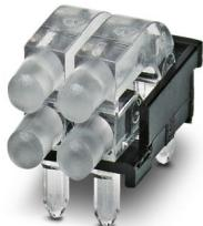
Multiple light guides with glare protection, passive, rigid, Raised head, conical, emission surface: spherical, number of displays: 4, (2 rows, 2 columns), pitch: 2.54 mm, ESD protection: <8 kV, can be used for the ME, ME-MAX, ME-IO, ME PLC, and EH housing ranges (housing must be processed)
