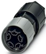
Connector, connection method: IDC connection, number of positions: 4+PE, 2.5 mm<sup>2</sup> ... 6 mm<sup>2</sup>, 690 V, 40 A, PA, black, with QUICKON nut, external cable diameter: 9 mm ... 14 mm
