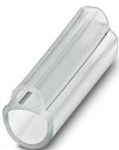
Conductor marker carrier, transparent, unmarked, cable diameter range: 0.6 ... 1.2 mm, mounting type: slide-on, text field height: 4 mm, text field width: 15 mm
