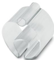
Conductor marker carrier, transparent, unmarked, cable diameter range: 14 ... 22 mm, mounting type: slide-on, text field height: 4 mm, text field width: 15 mm
