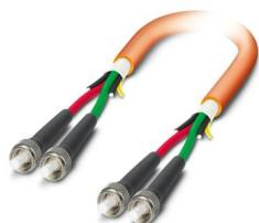
Robust PCF installation cable for indoor use with highly tear-proof aramid strain relief elements. Individual elements made from highly flexible FRNC material. The cable is halogen-free, ozone and UV-resistant with robust polyurethane (PUR) outer sheath, assembled with 2x F-SMA to 2x F-SMA, length: 1.5 m
