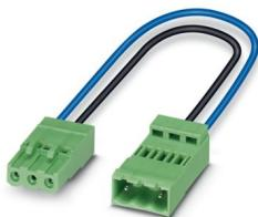
Assembled PCB connector / Connecting cable with 2 printed circuit board connectors, rated current: 9 A, Head 1: 3-position, pitch: 5.08 mm, Crimp connection, Pin, Cable 1: cable length: 0.38 m, Color: black, blue, Cable type: mPPE litz wire, Head 2: 3-position, pitch: 5.08 mm, product feature: PCB connectors for Smart Meter Gateways (SMGW), mPPE litz wire
