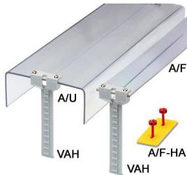
Flat-ribbon cover, for covering terminal strips, 2 mm thick, 2.5 cm wide, an additional requirement are 2 E/UK end brackets and 2 adjustable VAH cover holders. The max. supply length is 100 cm
