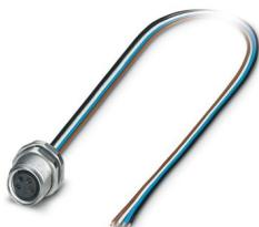
Device connector rear mounting, 4-position, A-coding, on free cable end, Individual wires, cable length: 1.2 m, 0.25 mm<sup>2</sup>, PVC litz wire
