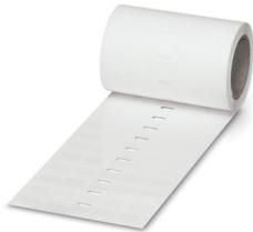
Label for rough surfaces, Roll, white, unmarked, can be labeled with: THERMOMARK E.300 (D)/600 (D), THERMOMARK ROLL 2.0, THERMOMARK ROLL, THERMOMARK ROLL X1, THERMOMARK ROLLMASTER 300/600, THERMOMARK X1.2, mounting type: adhesive, Number of individual labels: 1000, text field height: 17.8 mm, text field width: 50.8 mm
