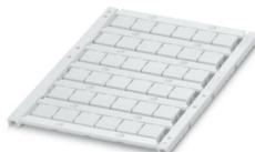
Marker for terminal blocks, Sheet, white, unmarked, can be labeled with: BLUEMARK E.CARD, BLUEMARK ID COLOR, BLUEMARK ID, BLUEMARK CLED, THERMOMARK PRIME 2.0, THERMOMARK PRIME, THERMOMARK CARD 2.0, THERMOMARK CARD, TOPMARK NEO, TOPMARK LASER, mounting type: latching, for terminal block width: 10.2 mm, Number of individual labels: 36, text field height: 9.6 mm, text field width: 8.9 mm
