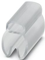
Conductor marker carrier, transparent, unmarked, cable diameter range: 4 ... 7 mm, mounting type: slide-on, text field height: 4 mm, text field width: 12 mm
