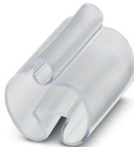
Conductor marker carrier, transparent, unmarked, cable diameter range: 10 ... 14 mm, mounting type: slide-on, text field height: 4 mm, text field width: 23 mm
