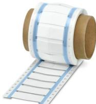
Shrink sleeve, Roll, white, unmarked, can be labeled with: THERMOMARK E.300 (D)/600 (D), THERMOMARK ROLLMASTER 300/600, THERMOMARK ROLL X1, THERMOMARK ROLL, THERMOMARK ROLL 2.0, THERMOMARK W, THERMOMARK X1.2, cable diameter range: 4.2 ... 12.7 mm, perforated, mounting type: slide-on, Number of individual labels: 500, text field height: 20 mm, text field width: 30 mm
