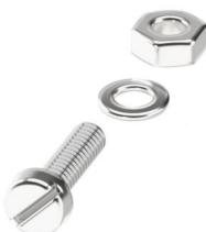
Screw set, for securing the header to the housing wall, consists of M2 x 8 screw, spring washer and nut, 1 piece each
