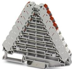
Marshalling panel, without actuating push button, nom. voltage: 250 V, nominal current: 8 A, connection method: Push-in connection, 1st, 2nd, 3rd, 4th, 5th, 6th, 7th and 8th level, Rated cross section: 1.5 mm<sup>2</sup>, cross section: 0.14 mm<sup>2</sup> - 2.5 mm<sup>2</sup>, mounting: NS 35/7,5, NS 35/15, color: gray, color of connection elements: red, white
