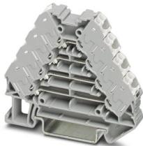
Marshalling panel, without actuating push button, nom. voltage: 250 V, nominal current: 10 A, connection method: Push-in connection, 1st, 2nd, 3rd and 4th level, Rated cross section: 1.5 mm<sup>2</sup>, cross section: 0.14 mm<sup>2</sup> - 2.5 mm<sup>2</sup>, mounting: NS 35/7,5, NS 35/15, color: gray, color of connection elements: white
