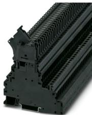
Fuse modular terminal block, fuse type: Glass / ceramics / ..., fuse type: G / 5 x 20, nom. voltage: 250 V, Thermal continuous current  $I_{th}$ : 28 A, connection method: Screw connection, Rated cross section: 4 mm<sup>2</sup>, cross section: 0.14 mm<sup>2</sup>- 6 mm<sup>2</sup>, connection method: Screw connection, Rated cross section: 4 mm<sup>2</sup>, cross section: 0.14 mm<sup>2</sup>- 6 mm<sup>2</sup>, mounting type: NS 35/7,5, NS 35/15, color: black
