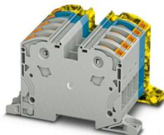
High-current terminal block, Blocked, nom. voltage: 1000 V, nominal current: 125 A, number of connections: 10, number of positions: 5, connection method: PowerTurn connection, Rated cross section: 35 mm<sup>2</sup>, cross section: 2.5 mm<sup>2</sup> - 35 mm<sup>2</sup>, mounting type: direct screw connection, color: gray/blue/black-yellow
