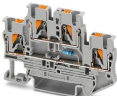
Component terminal block, 1st and 2nd level, connection method: Push-in connection, Rated cross section: 2.5 mm<sup>2</sup>, cross section: 0.14 mm<sup>2</sup> - 4 mm<sup>2</sup>, mounting: NS 35/7,5, NS 35/15, color: gray
