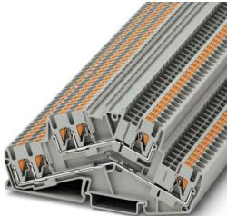
Double-level terminal block, nom. voltage: 800 V, nominal current: 20 A, connection method: Push-in connection, 1st and 2nd level, Rated cross section: 2.5 mm<sup>2</sup>, cross section: 0.14 mm<sup>2</sup> - 4 mm<sup>2</sup>, mounting type: NS 35/7,5, NS 35/15, color: gray
