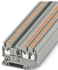
Component terminal block, with integrated 1N4007 diode, nom. voltage: 800 V, nominal current: 0.5 A, number of connections: 3, connection method: Push-in connection, Rated cross section: 2.5 mm<sup>2</sup>, cross section: 0.14 mm<sup>2</sup> - 4 mm<sup>2</sup>, mounting type: NS 35/7,5, NS 35/15, color: gray
