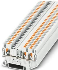
Feed-through terminal block, nom. voltage: 800 V, nominal current: 24 A, number of connections: 3, connection method: Push-in connection, Rated cross section: 2.5 mm<sup>2</sup>, cross section: 0.14 mm<sup>2</sup> - 4 mm<sup>2</sup>, mounting type: NS 35/7,5, NS 35/15, color: white
