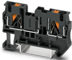
Fuse modular terminal block, fuse type: Blade, fuse type: ISO 8820-3 Type F (miniature), nom. voltage: 400 V, nominal current: 10 A, connection method: Push-in connection, Rated cross section: 4 mm<sup>2</sup>, cross section: 0.2 mm<sup>2</sup>- 6 mm<sup>2</sup>, mounting type: NS 35/7,5, NS 35/15, color: black
