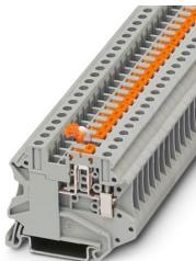
Knife-disconnect terminal block, With test socket screws for insertion of test plugs, nom. voltage: 500 V, nominal current: 20 A, connection method: Screw connection, Rated cross section: 2.5 mm<sup>2</sup>, cross section: 0.14 mm<sup>2</sup> - 6 mm<sup>2</sup>, mounting: NS 35/7,5, NS 35/15, color: gray
