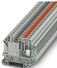
Knife-disconnect terminal block, with actuation latch, nom. voltage: 500 V, nominal current: 20 A, connection method: Screw connection, Rated cross section: 6 mm<sup>2</sup>, cross section: 0.2 mm<sup>2</sup> - 10 mm<sup>2</sup>, mounting: NS 35/7,5, NS 35/15, color: gray
