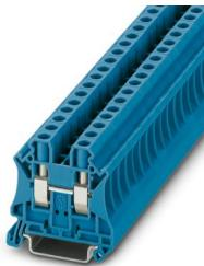
Feed-through terminal block, nom. voltage: 1000 V, nominal current: 41 A, number of connections: 2, connection method: Screw connection, Rated cross section: 6 mm<sup>2</sup>, cross section: 0.2 mm<sup>2</sup> - 10 mm<sup>2</sup>, mounting type: NS 35/7,5, NS 35/15, color: blue
