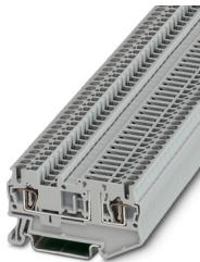
Disconnect terminal block, Current and voltage are determined by the plug used., nom. voltage: 400 V, nominal current: 20 A, connection method: Spring-cage connection, Rated cross section: 2.5 mm<sup>2</sup>, cross section: 0.08 mm<sup>2</sup> - 4 mm<sup>2</sup>, mounting: NS 35/7,5, NS 35/15, color: gray
