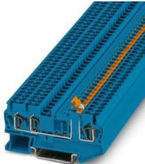
Knife-disconnect terminal block, nom. voltage: 400 V, nominal current: 20 A, connection method: Spring-cage connection, Rated cross section: 2.5 mm<sup>2</sup>, cross section: 0.08 mm<sup>2</sup> - 4 mm<sup>2</sup>, mounting: NS 35/7,5, NS 35/15, color: blue
