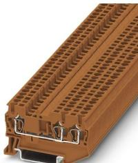
Feed-through terminal block, nom. voltage: 800 V, nominal current: 24 A, number of connections: 3, connection method: Spring-cage connection, Rated cross section: 2.5 mm<sup>2</sup>, cross section: 0.08 mm<sup>2</sup> - 4 mm<sup>2</sup>, mounting type: NS 35/7,5, NS 35/15, color: brown
