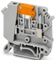
Knife-disconnect terminal block, With test socket screws for insertion of test plugs, nom. voltage: 500 V, nominal current: 16 A, Thermal continuous current  $I_{th}$ : 16 A, connection method: Screw connection, Rated cross section: 4 mm<sup>2</sup>, cross section: 0.2 mm<sup>2</sup> - 6 mm<sup>2</sup>, mounting: NS 35/7,5, NS 35/15, NS 32, color: gray
