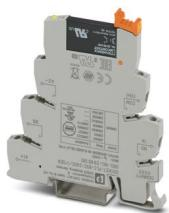
PLC-INTERFACE for input functions, consisting of PLC-BSC.../SEN basic terminal block with screw connection and plug-in miniature solid-state relay, for mounting on DIN rail NS 35/7,5, 1 N/O contact, input: 24 V DC, output: 3 - 48 V DC/100 mA
