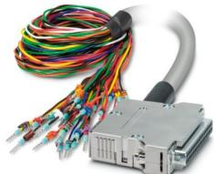
Assembled shielded round cable; connection 1: Twisted pair (37-position) (The wires are marked and fitted with ferrules); connection 2: D-SUB socket strip (1x 37-position); cable length: 1 m
