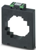
Window-type current transformer, 1600 A AC primary current; 1 A AC secondary current; accuracy class 1; 10 VA rated power
