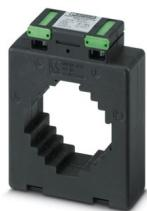
Window-type current transformer, 1250 A AC primary current; 1 A AC secondary current; accuracy class 1; 2.5 VA rated power
